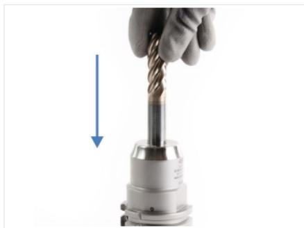
Fig. 7: Inserting tool
