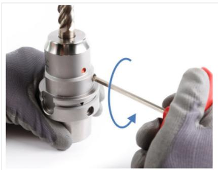
Fig. 12: Loosening clamping screw
