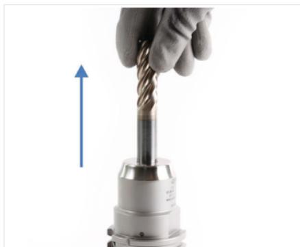
Fig. 13: Removing tool
