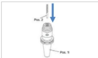
Figure 5: Inserting tool
